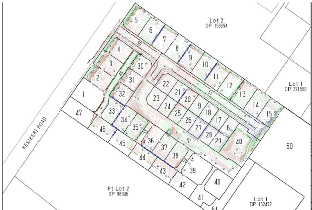
Figure C - As-Built Earthworks drawings (Source: Sheet 02, EWA16655 R&B Drawings). Green and blues indicate the extent of fill, and oranges and red excavation. Blue lines show the location of the Magnum stone retaining walls.
